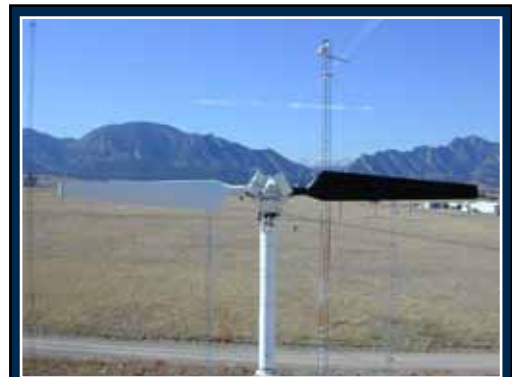
NREL-DOE Wind Turbine, with Aeroprobes Mounted on Black Blade (Photo Courtesy NREL)
