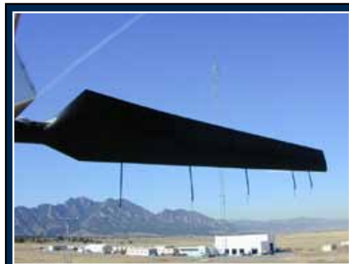
Five Aeroprobes Mounted on Instrumented NRELDOE Rotor Blade (Photo Courtesy NREL)
