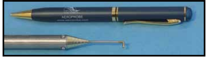
Fast-Response Drilled Elbow Probe for Turbine Application. Embedded Sensors Are Located at Cross-Section beneath Screws
