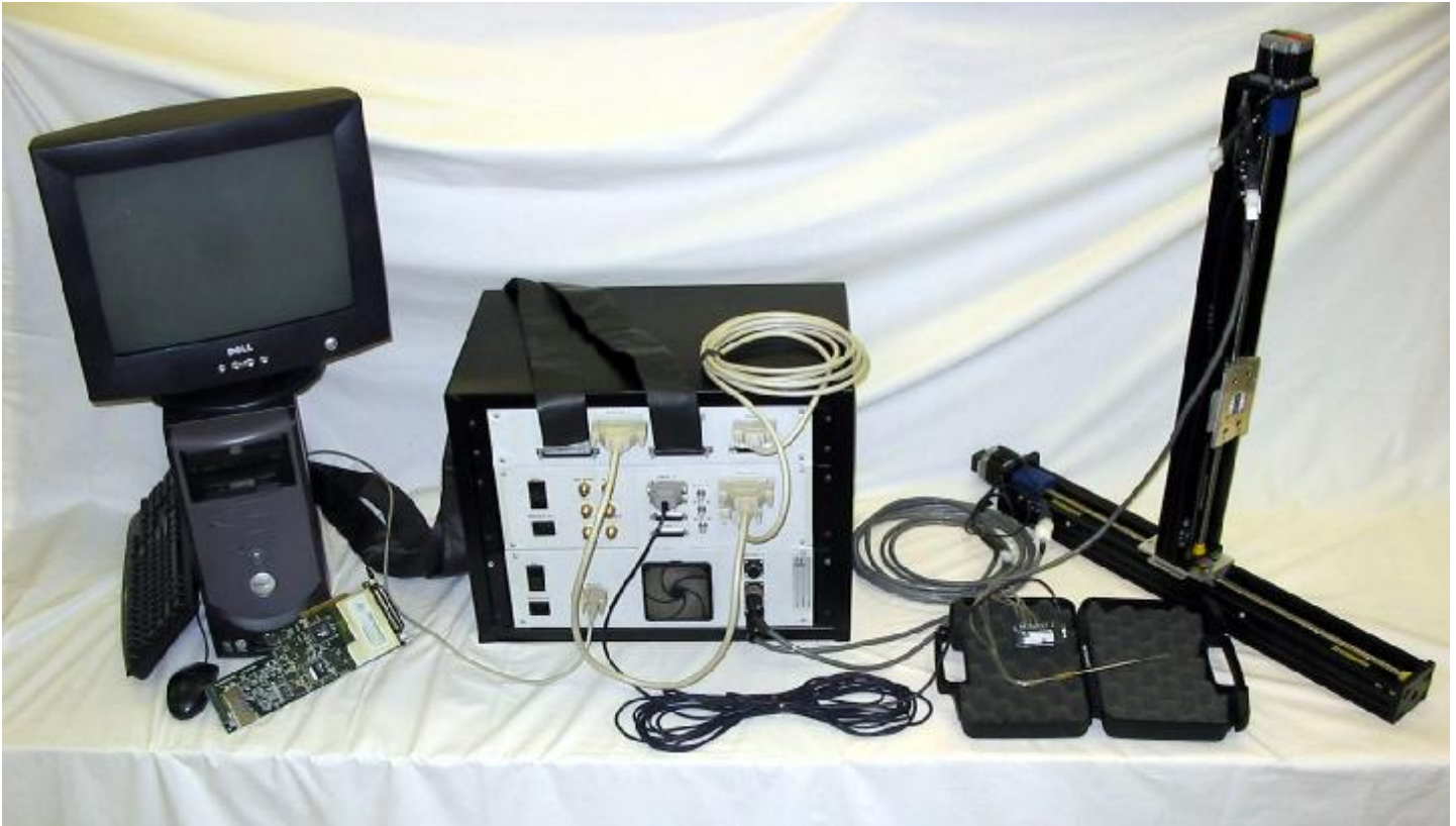
Aeroprobe System with Conventional Probe and Pressure Scanner
